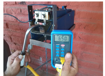
Pyrometer indicating proper blade temperature of 650°C.
